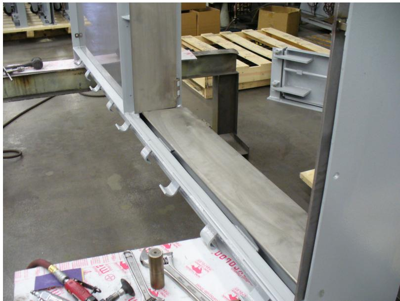
*Barrier from the front in open position – note side cover panels to conceal sliding panel*
