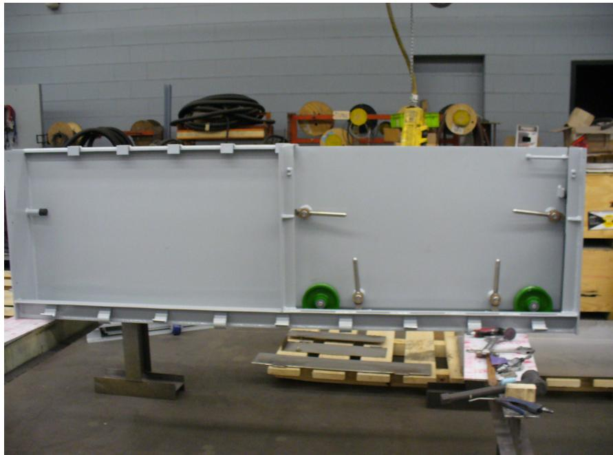
*Barrier from the back in the closed (sealed position) – note panel cover to the left designed to hide sliding panel when not in use*
